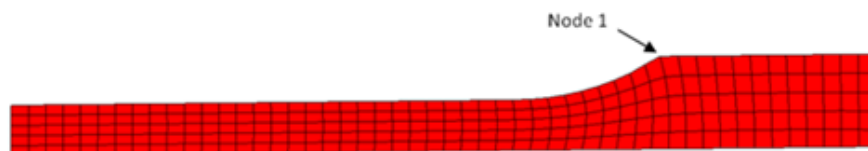
Geometry of the Tensile Specimen (One Quarter of the Specimen is Modeled)
