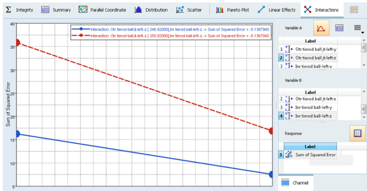
Controlled design variable plot for "Otr_tierod_ball_jt-left-z" & "Inr_tierod_ball_jt-left-z" interaction
