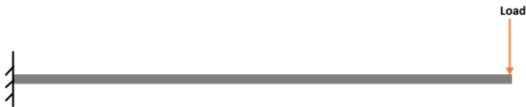
Cantilever beam under end load condition
