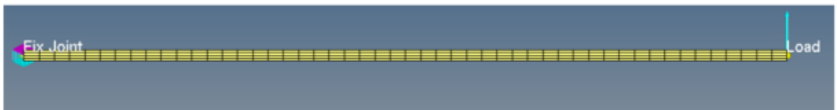
Cantilever beam with end load
