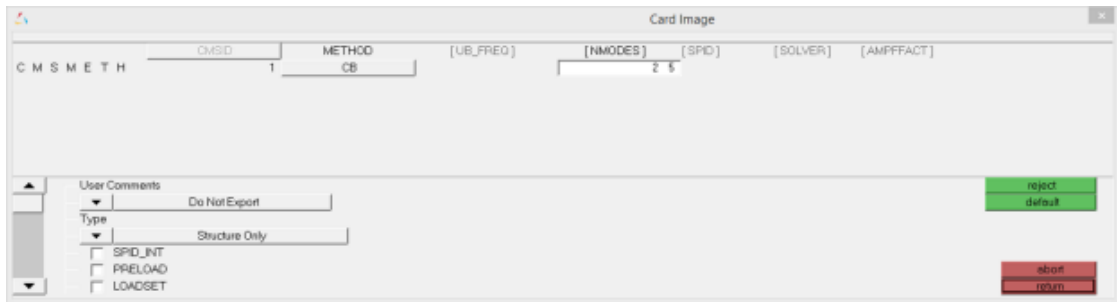
CMS load collector card image dialog with method specified as Craig-Bampton (CB) and the number of modes as 25
