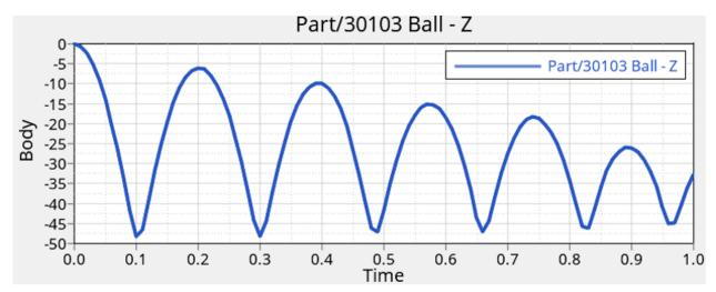
We can also plot the penetration distance for this flexible contact.
