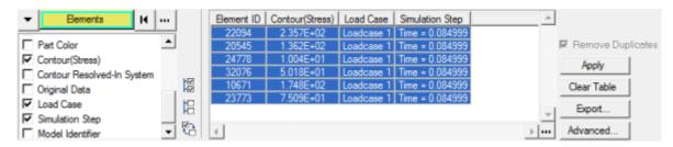
Observe the table in the panel shows the element ID, the corresponding contour value, the load case, and the simulation step for each of the selected elements.
