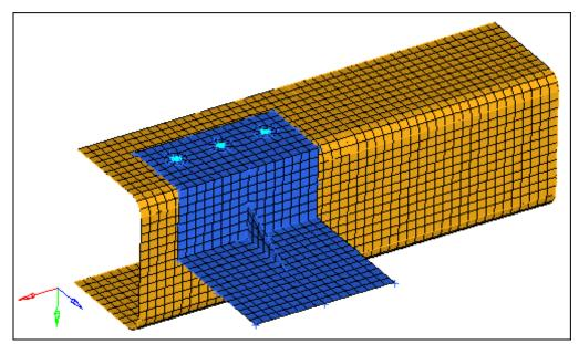
The model contains the bracket and channel assembly in the following image.
