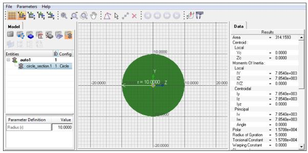
HyperBeam module with the standard solid circle section
