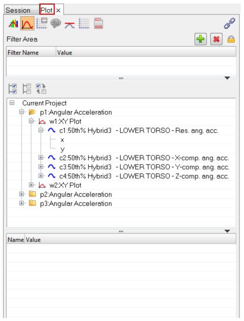
The **Plot Browser** can be turned on or off using the **View > Browsers > HyperGraph 2D > Plot** menu options. A check mark indicates that the HyperGraph 2D Plot Browser is activated for display in the Tab Area.
