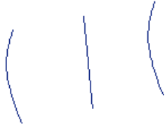
Figure 1578: Lines used to define a skinned surface.
