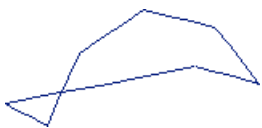
Figure 1576: Creating a surface with these lines results in a relatively complex surface.
