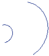
Figure 1580: Lines used to create a ruled surface.
